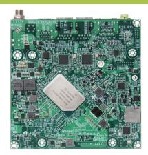
Intel Atom® Dual/Quad-core x6000E family SoC (up to 12W)
