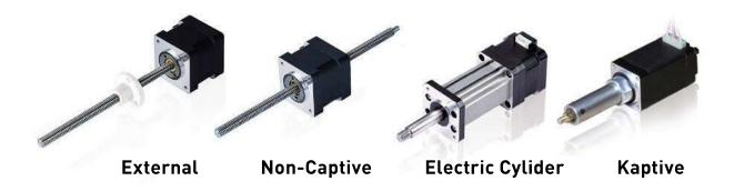
DINGS' offers a unique line of stepper motor linear actuators that open new avenues for equipment designers that require high performance and endurance in a small package. The various products convert the rotational movement of a stepper motor to linear motion, with the use of a lead screw and an engineered thermoplastic nut (Delrin). This allows linear actuators to provide quiet, efficient, durable and cost effective linear motion solutions.
